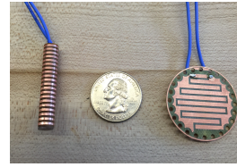
Figure 8. Electrodes for two variations of Keppi V3
