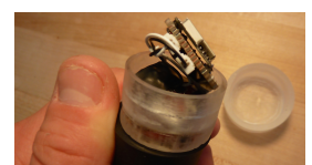
Figure 6. Electronics outside the housing connected to the FSR
