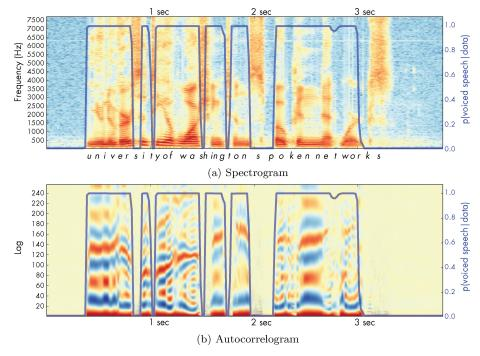
Fig. 4. Inferred voicing posterior (blue line, right y axis) overlayed on examples from Figure 2.
